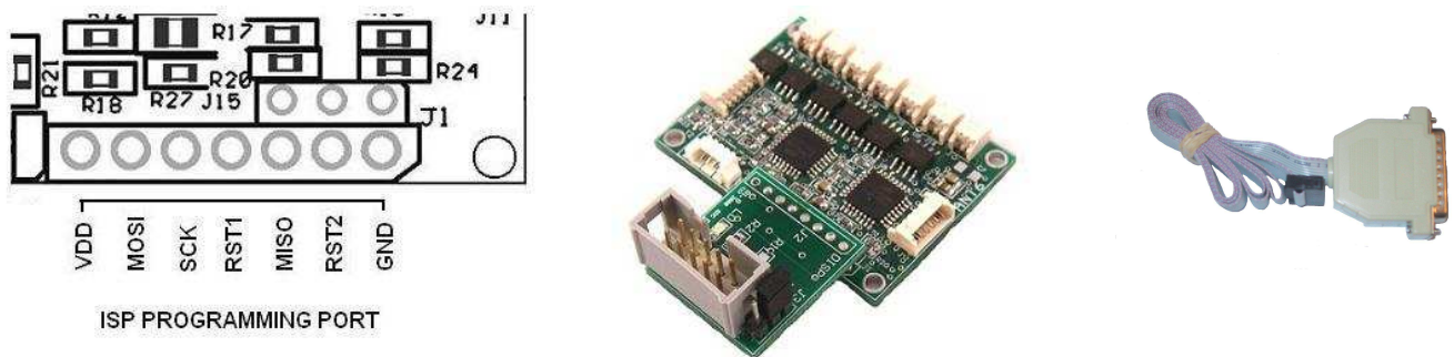
Figure 3-2. SPI/Programming Port J1 and ISP10 Programming Adapter.
