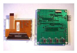
Flip the screen over and position the ribbon cable close to the connector – make sure the securing tabs are pulled back away from the connector.
