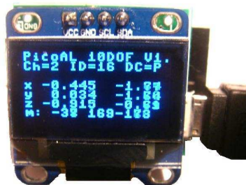
OLED 128x64 pixel display mounted on PicoA
