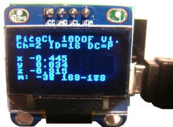
OLED 128x64 pixel display mounted on PicoC
