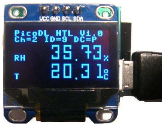
OLED 128x64 pixel display mounted on PicoD.
