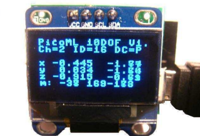
OLED 128x64 pixel display mounted on PicoM
