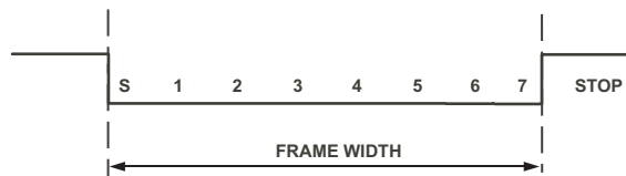
Figure 15-21. Autobaud Detection Character 0x00
